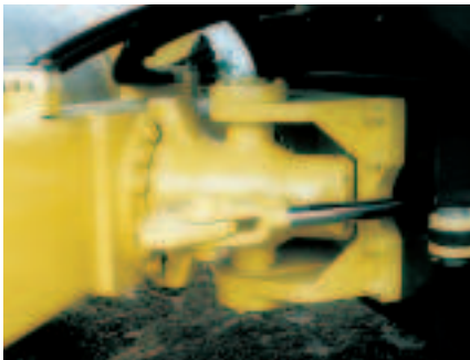
Bolt-on oscillating, articulation joint for long life and servicing ease
