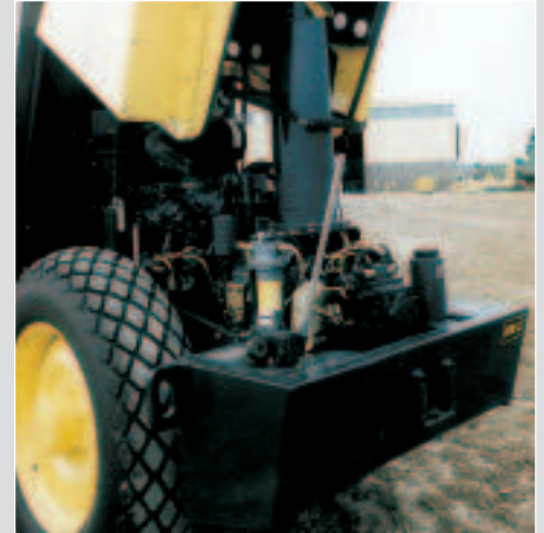
Wide opening hood provides easy access to all components
